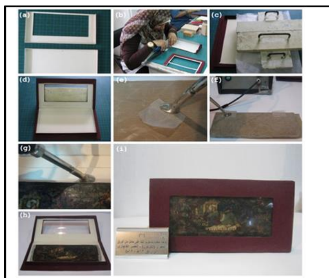
Figure 10. Steps of making the storage box and the final display, (a) (b) (c) step by step making the box, (d) the final box, (e) (f) (g) adhering the painting in the box with a sheet of Japanese paper and polyethylene, (h) (i) final display.
