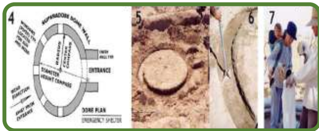
Figure 5: The picture represents the location of the door in the plan in relation to the direction of the wind, the foundations and the method of stacking and packing Source: https://syrianchange.wordpress.com
