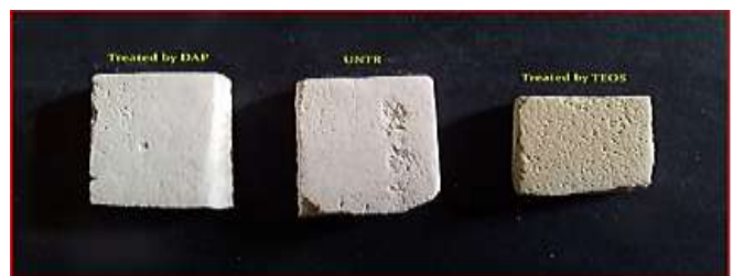
Fig. 11. Effect of consolidants on the appearance of treated samples compared to the reference sample (UNTR).
