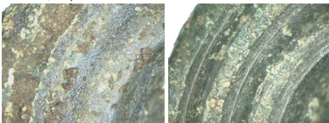
(Figure 6) Cleaning results for Object 4: (left) laser-cleaned surface (right) mechanically cleaned surface [Capucine Korenberg and Alexandra Baldwin.,2006]
