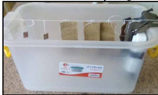
Figure 2. Hanging the textiles and bronze samples by thermal thread
